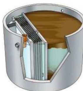
Figure 13 : Micro station à culture fixée (EPUR®)
